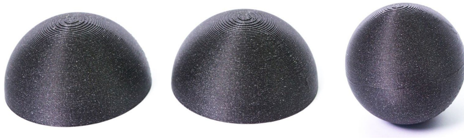
Pict. 29 - A sphere printed in two separate parts glued together
