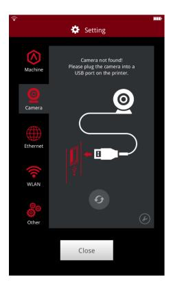
Select the camera and wait for the connection. Pictures can be viewed on RaiseTouch and ideaMaker after successfully connected.
