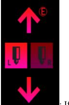
: If the machine is a dual-nozzles machine, click the left and right nozzle to switch the nozzles.
