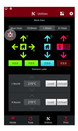
The Utilities interface consists of two functional modules, Move Axes and Load & Unload. The height of the X.Y axis and the hot bed can be located by manually entering the moving distance. Material can be replaced by load and unload.
