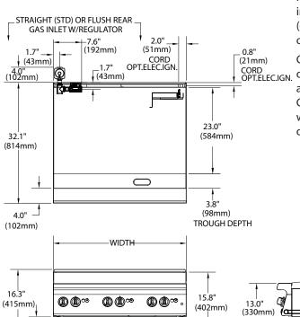
For use with Natural or Propane gas only. Gas input ratings shown for installations up to 2000 ft., (610m), above sea level. Please specify altitudes over 2000 ft. and gas type required when ordering.
