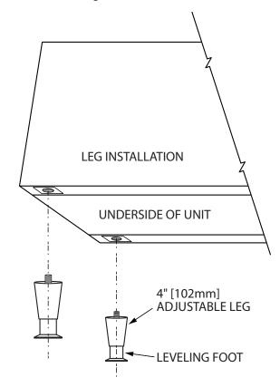
Level the appliance by adjustment of leveling bolts or legs. Use a spirit level and check for level four ways; across front and back, then down left and right edges. Level any adjacent units to the first. A griddle may not rest evenly on the appliance body if it is not properly leveled.
