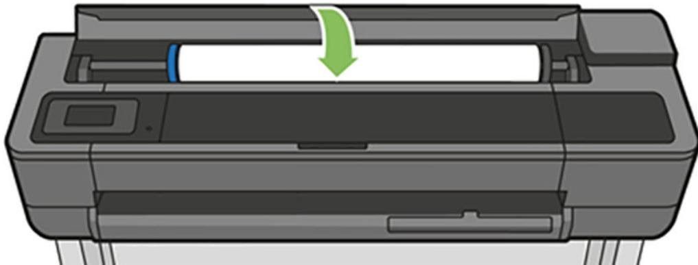
11. Reload the roll, or load a new sheet; see [Paper handling on page 31](#).
