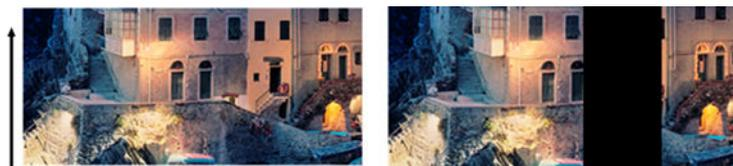
Original Scan affected by a failing scanbar
