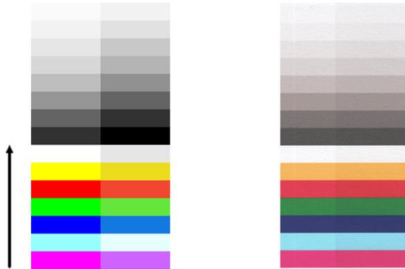
Sometimes the color mismatch between adjacent modules can be enormous, showing a serious scanner malfunction, as in the following example. If this occurs, see [Completely wrong colors on page 162](#).
