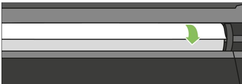
6. Roll the paper into the printer until you feel resistance and the paper flexes slightly. When the printer detects the paper, it beeps, and feeds in the paper automatically.
