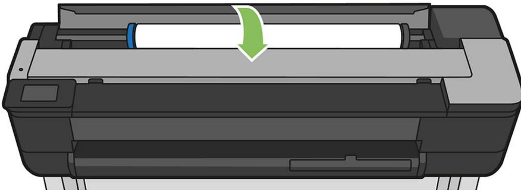
11. Reload the roll, or load a new sheet; see [Paper handling on page 31](#).
