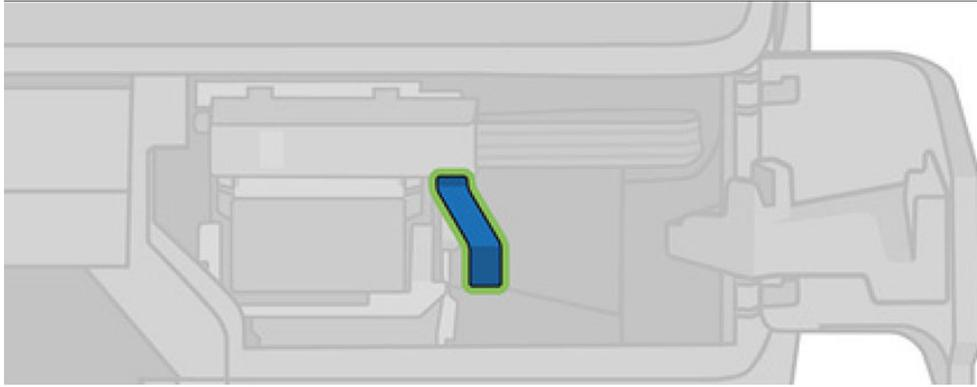
6. Raise the blue lever to release the tube connector and store the tubes connector on the tubes connector holder in the printer door.
